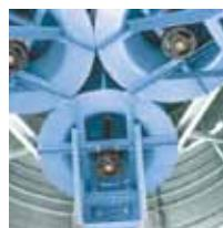
**14.** Internally assembled tubular centrifugal ventilators provide high-volume air flow to drying section as well as high absorption rate for cooling section.
