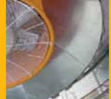
**8.** Conic separation of Drying and Cooling sections prevents foreign substance accumulation and provides easy maintenance and cleaning.
