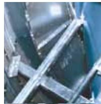
**12.** Conic separation of Drying and Cooling sections prevents foreign substance accumulation and provides easy maintenance and cleaning.
